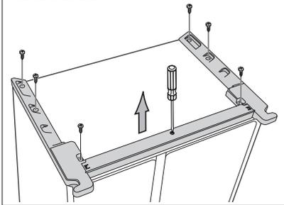
2. Remove hinge screws **3** and the ground screw **4** by turning counter-clockwise, and take off the upper hinge **5**. Be careful that the door does not fall on you as you are removing it.
