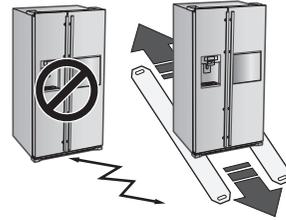
First things first! Make sure that you can easily move your refrigerator to its final location by measuring doorways (both width and height), thresholds, ceilings, stairways, etc. The following chart details the exact height and depth.
