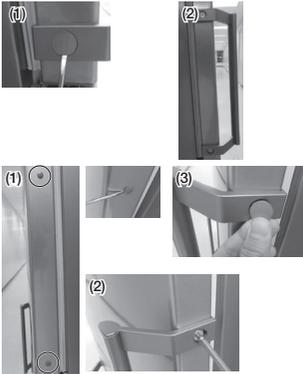
Remove the Cap by Flat-Head (-) screwdriver and assemble the Handle and Cap-Handle.
