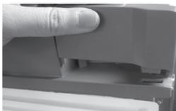
23. Insert the Cover Wire Door on the top of Fridge door and then push it to assemble completely. Check the wire position that should be located the back side of Cover Wire Door.
