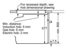
measurements in mm
