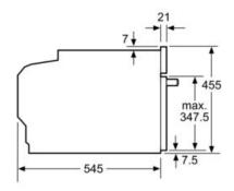
measurements in mm
