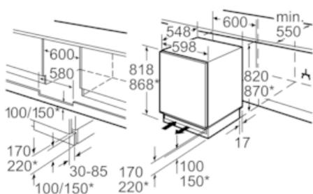
\* variable base/substructure height
