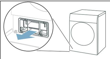
4. Remove all of the fluff from the heat exchanger cover and remove the fluff filter.
