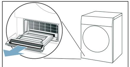
**Note:** The fluff collector may contain fluff and residual water, which may drip out of it when you pull it out.
