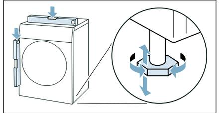
3. If necessary, turn the appliance feet to make sure it is level. You can now connect the appliance.
