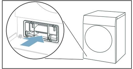
**Note:** You can only slide the heat exchanger cover in if the fluff collector is in the appliance.
