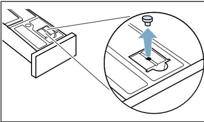
2. Turn the condensation container 180° onto its underside and insert the stopper.
