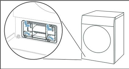
3. Pull the heat exchanger cover out by its grip.
