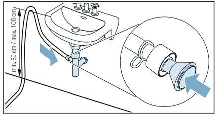
The connection point must be secured using a hose clamp (12-22 mm clamping range, available from specialist retailers). When connecting to a siphon, make sure that the drain hose is routed at a height of at least 80 cm, but no more than 100 cm.
