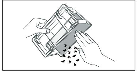
**Note:** Ensure that no dirt remains on the seals of the heat exchanger cover.
