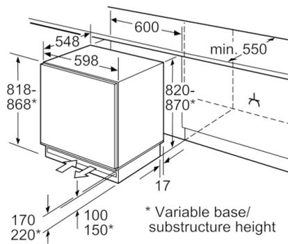
Space for electrical connection next to the appliance on the left or right-hand side.
