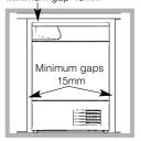
If you are going to install the appliance under a work counter, be sure to leave a 10mm space between the top and any other objects on or above the machine and a 15mm space between
