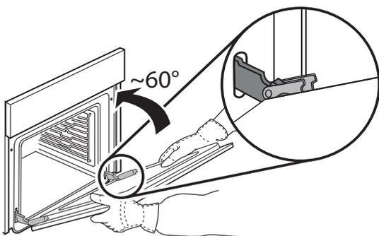
4. Take a firm hold of the door with both hands – do not hold it by the handle. Simply remove the door by continuing to close it while pulling it upwards at the same time until it is released from its seating.
