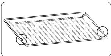
Insert the wire rack into position with the protruding parts (stoppers on both sides) towards the front so that the wire rack supports the rest position for large loads.
