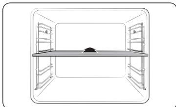
Insert the divider in level 3 to separate the cooking chamber in two compartments. The oven senses the divider and activates the upper compartment by default.
