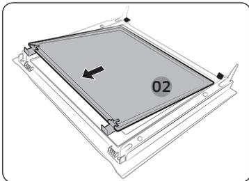
4. Remove the second sheet from the door in the arrow direction.
