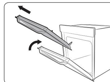
2. Close the door approximately 70°. Hold the oven door by the sides using both hands, and lift and pull upwards until the hinges are removed.
