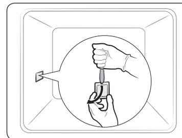
1. Hold the lower end of the cover of the side oven light with one hand, and use a flat-sharp tool such as a table knife to remove the cover as shown.
