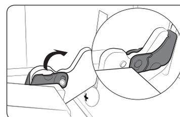
4. When done, follow steps 1 to 2 above in the reverse order to reinstall the door. Make sure the clips are hinged on both sides.
