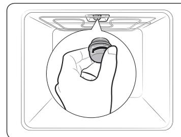
1. Remove the glass cap by turning anti-clockwise.
