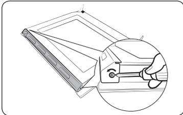
1. Use a screwdriver to remove the screws on the left and right sides.
