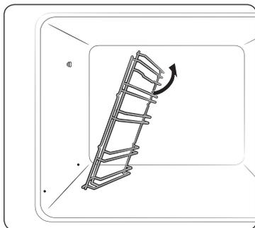
2. Pull and remove the bottom line of the left side runner.
