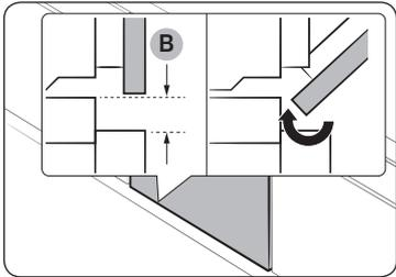
Secure at least 3 mm of gap **(B)** so that the door opens and closes smoothly.
