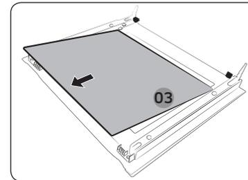
5. Remove the third sheet from the door in the arrow direction.
