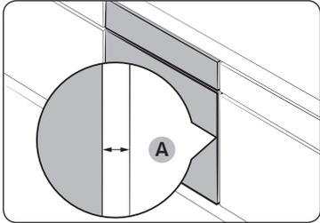
Make sure to leave a gap **(A)** of at least 5 mm between the oven and each side of the cabinet.
