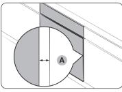
Make sure to leave a gap **(A)** of at least 5 mm between the oven and each side of the cabinet.
