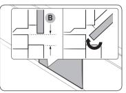
Secure at least 3 mm of gap **(B)** so that the door opens and closes smoothly.
