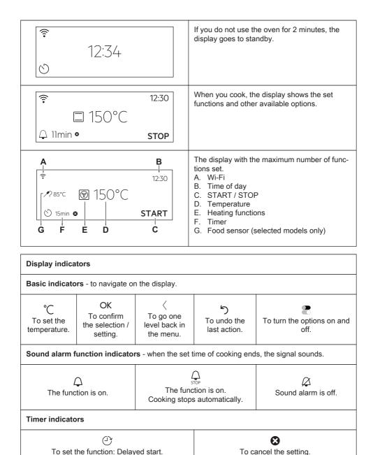
Wi-Fi indicator - the oven can be connected to Wi-Fi.
