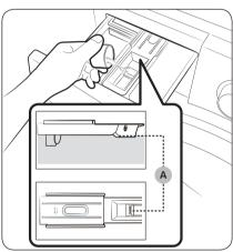
Apply fabric softener to the Softener compartment. Do not exceed the max line (A). Softener is dispensed into the wash during the final rinse.
