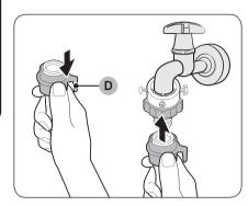
While pulling down part (D) on the water hose, connect the water hose to the adaptor. Then, release part (D). The hose fits into the adaptor with a clicking sound.
