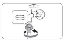
1. Connect the water hose to the water tap, and then turn the connector clockwise as shown.
