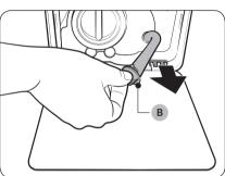
Put an empty, spacious container around the cover, and stretch the emergency drain tube to the container while holding the tube cap (B).
