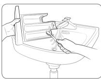
**3.** Clean the drawer components in flowing water using a soft brush.
