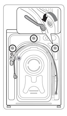
1. Locate the shipping bolts (marked with circle in the figure) on the rear side of the washing machine.
