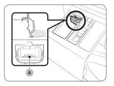
First insert the provided liquid container in the **1** mainwash compartment. Then, apply liquid detergent to the container below the marked max line (A).
