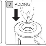
Add additional ingredients in to the blender through the filler cap aperture. Do not do this when blending warm items.
