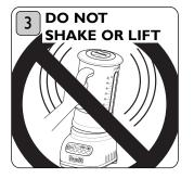
Whilst blending do not shake or lift off the jar. If the motor is running this will permanently damage the drive coupling.
