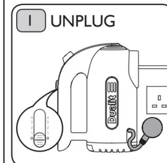
To protect your hand mixer, it is fitted with an overheat cut-out, which will automatically stop the handmixer if overloaded. **If this happens, turn the speed control to '0', unplug and eject attachments.**
