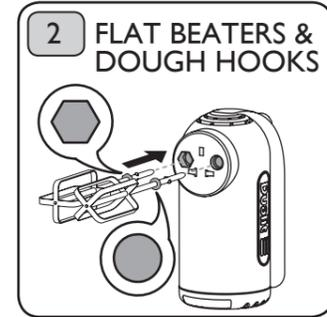
Ensure you insert the correct beater into the correct hole. Match the shape on the underside of the mixer to the shape on the attachment stem. Insert with a slight twist and push action until they click in to place.
