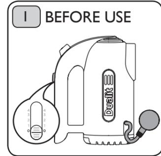
Before handling the beaters, or balloon whisk, ensure the mixer is unplugged from the electrical outlet and the speed control switch is set to the '0' position.
