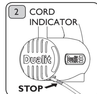
To prevent cord damage always pull power cord out gently. If the cord jams, rotate the swivel base counter clockwise half a turn, then pull out the cord. Do not pull cable past the red indicator on the power cord.
