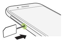
When inserting the eject tool into the tray eject hole to remove the card tray, do not obstruct the tray to avoid damaging the eject mechanism inside the slot.
