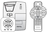
Press  $\blacksquare / \blacksquare$  on the projector or remote control to display the 2D Keystone page. Press  $\blacktriangle / \blacksquare$  to adjust vertical values from -30 to 30. Press  $\blacktriangleleft / \blacktriangleright$  to adjust horizontal values from -30 to 30.
