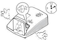
Never replace the lamp assembly or any electronic components unless the projector is unplugged.
