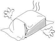
If the ventilation holes are seriously obstructed, overheating inside the projector may result in a fire.
