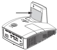
Remove dust with a "Bellows/Lens Blower" readily available from Camera shops to prevent scratching the mirror when subsequently wiped.
