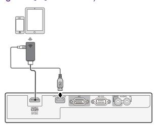
Connect the dongle to HDMI and USB TYPE-A ports on the projector and switch the input signal to HDMI I.
