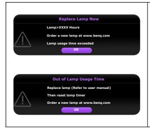
The lamp MUST be replaced before the projector will operate normally.
