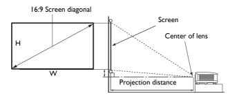
• The screen aspect ratio is 16:9 and the projected picture is in a 16:9 aspect ratio
