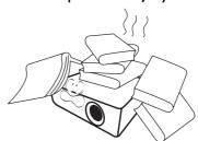
16. When the projector is under operation, you may sense some heated air and odor from its ventilation grill. It is a normal phenomenon and not a product defect. 17. Do not place liquids near or on the projector. Liquids spilled into the projector may cause it to fail. If the projector does become wet, disconnect it from the power supply's power outlet and call BenQ to have the projector serviced.
