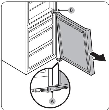
8. With the freezer door sitting on the **bottom hinge (A)**, slowly pull the **bottom hinge (A)** to remove it from the holder on the bottom of the refrigerator. Once the **bottom hinge (A)** is removed from the holder, remove it from the freezer door, and then pull the freezer door down to remove it from the **middle hinge (B)**.
