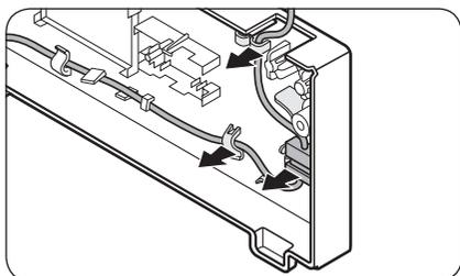
3. Remove the wire and the wire connector placed on the holder underneath the top cover.
