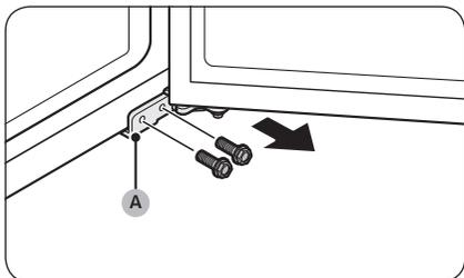
7. Open the freezer door, and then use a Phillips screwdriver to remove the screws fastening the **bottom hinge (A)**.
