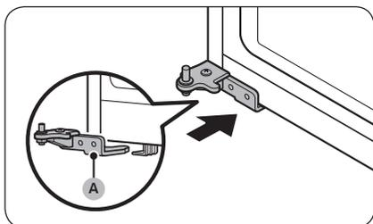
17. Turn the levelling leg on the opposite side of where **bottom hinge (A)** removed. Then, Put the **bottom hinge (A)** on the holder.
