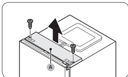
1. With the fridge door closed, use a Phillips screwdriver to remove the screws fastening the top cover (A).
