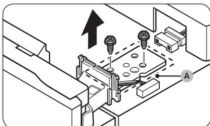
5. Use a socket wrench (8 mm) to remove the screws fastening the **top hinge (A)**.
