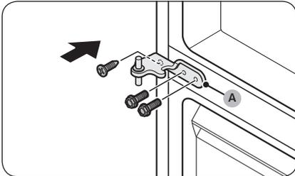
15. Fasten the **middle hinge (A)** to the opposite side of where it was removed.
