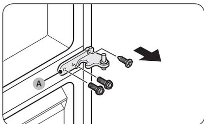
9. Use a Phillips screwdriver and socket wrench (10 mm) to remove the screws fastening the **middle hinge (A)**.
