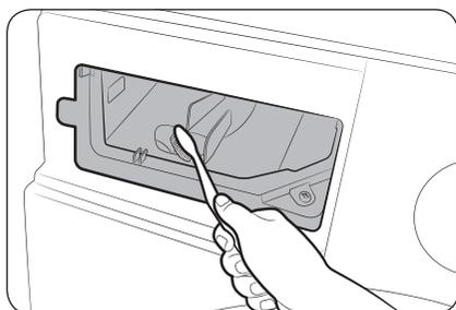
4. Clean the drawer recess using a bottle brush to remove detergent residues and limescale on the drawer recess.
