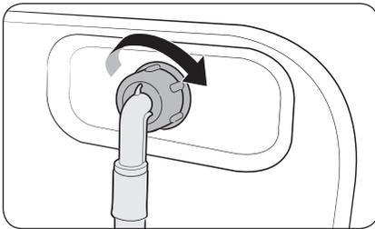
2. Connect the other end of the water hose to the inlet valve on the back of the washing machine. Turn the hose clockwise to tighten.
