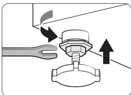
3. When levelling is complete, tighten the nuts using the spanner.
