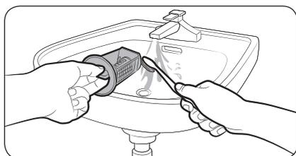
5. Clean the debris filter using soft brushes. Make sure the drain pump propeller inside the filter is unclogged.
