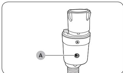
The aqua hose alerts users of a risk of water leaks. It senses the water flow and turns red on the centre indicator (A) in case of a leak.
