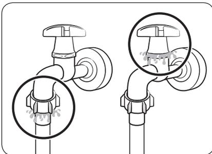
3. Open the water tap and check if there are any leaks around the connection areas. If there are water leaks, repeat the steps above.
