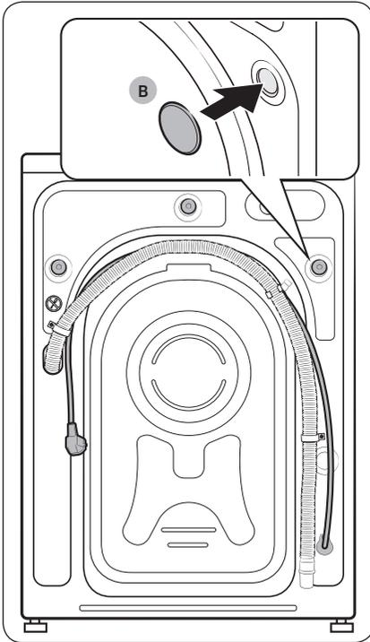
3. Insert the **bolt caps (B)** to the holes (marked with circle in the figure).
