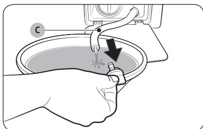
4. Open the tube cap and let water in the **emergency drain tube (C)** flow into the container.
