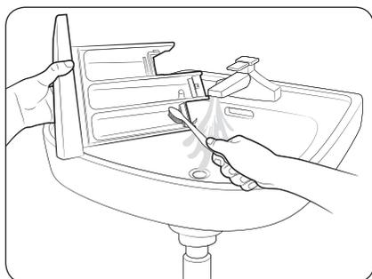
3. Clean the drawer components in flowing water using a soft brush.
