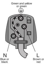
As the colours of the wires in the mains lead of this appliance may not correspond with the coloured markings identifying the terminals on your plug, proceed as follows:
