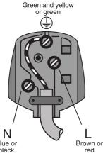
As the colours of the wires in the mains lead of this appliance may not correspond with the coloured markings identifying the terminals on your plug, proceed as follows:
