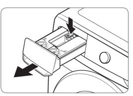
1. While holding down the **release lever** on the inner of the drawer, pull the detergent drawer to remove.
