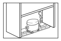
7. A special receptacle is supplied to store the mains plug during transit. The receptacle is fixed at the back of the cabinet, on the right hand side of the compressor. (See diagram) Gently remove the plug from the receptacle. Never pull the mains cord, you may damage the appliance. In the case of transportation, ensure you locate the plug in the receptacle provided to avoid transit damage.
