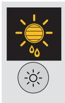
After selecting a programme that has a Sensor Dry Option, press and release the button until the required dryness sensing level is displayed. If the sensing option is not available the display will flash and the buzzer beeps three times.
