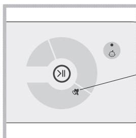
**! The water bottle/clean filter light comes on when you select a programme to remind you to make sure that the water bottle is empty and that the filter is clean before starting a new cycle'**
