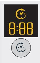
After selecting a Programme that has a Delay Start Option a delay start time can be selected. Each press of the Delay start button
