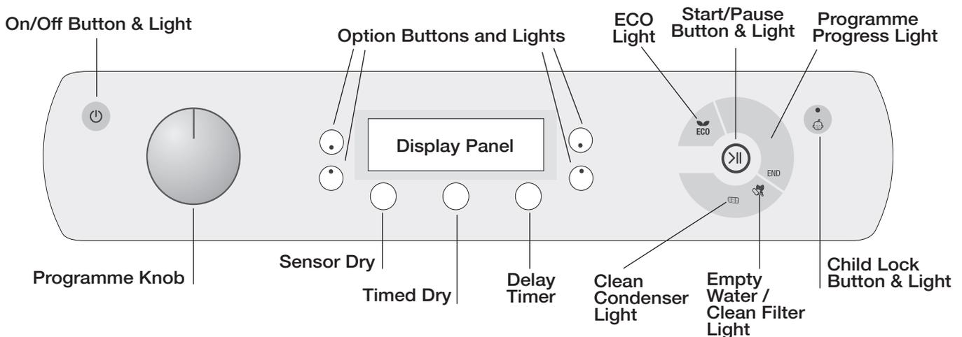
The **On/Off** button/ light
