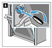
Left-hand lock: Anti-clockwise Right-hand lock: Clockwise
