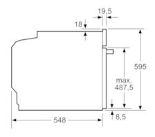
measurements in mm
