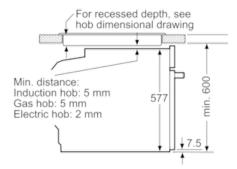
measurements in mm
