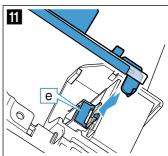
10. Insert the second reflector on the right-hand side in the same way as the left-hand reflector.
