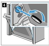
Left-hand lock: Anti-clockwise Right-hand lock: Clockwise
