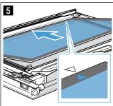
5. Push down on the intermediate panel around **b**, slide the holder c in at an angle and push down until it clicks into place (Fig. 6).
