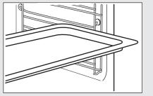
Wire shelf and deep pan together: Push the deep pan between the guide bars of the shelf support and the wire shelf on the guide bars above.
