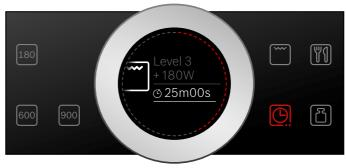
**6.** Press the start/stop button  $\triangleright$  to start. The cooking time counts down on the display.
