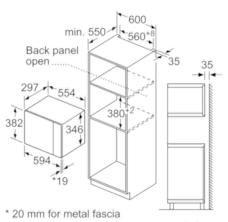
measurements in mm
