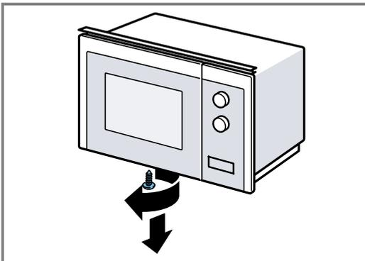
2. Remove the cover at the base of the microwave.
