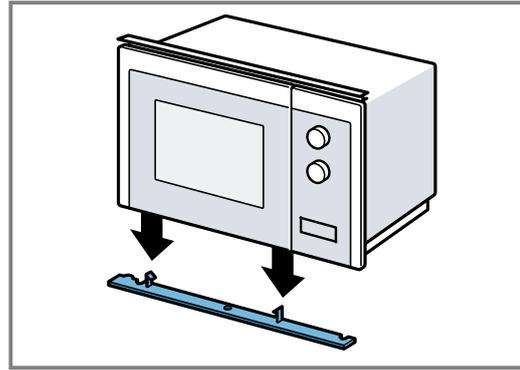
3. Screw the middle screw tightly on the base of the microwave.
