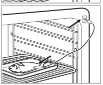
Insert the tip of Food Sensor exactly in the centre of the casserole. Food Sensor should be stabilized in one place during baking. Use a solid ingredient to achieve that. Use the rim of the baking dish to support the silicone handle of Food Sensor. The tip of Food Sensor should not touch the bottom of a baking dish. Cover Food Sensor with the remaining ingredients.
