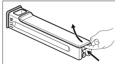
2. Remove the wave-breaker. Pull it away from the drawer body until it snaps out.
