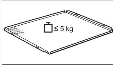
For rolls, brezels and small pastries. Suitable for steam functions. The discolouration of the surface has no effect on the functions.
