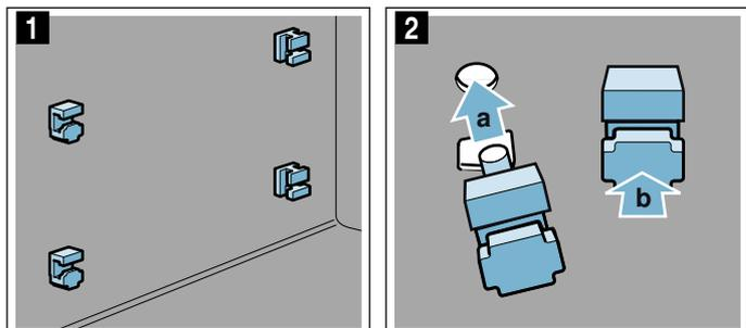
3. Use the hook to attach the rear holder into the upper hole **a** and push it into the lower hole **b** (fig. **3**).
