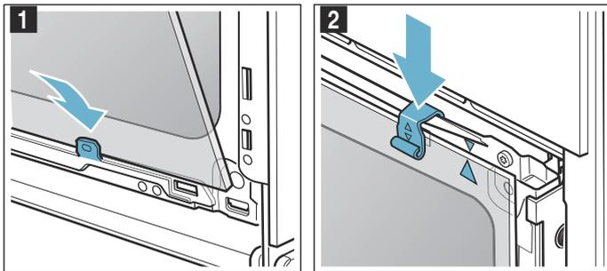
3. Insert the front panel downwards into the retainers (fig. 3).
