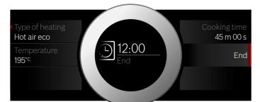
Press the > Start/Stop button to start. The time at which the appliance will start is shown in the display.
