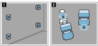
3. Use the hook to attach the rear holder into the upper hole **a** and push it into the lower hole **b** (fig. ☑).
