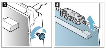
Push both retainers at the top of the intermediate panel upwards, but do not remove them (fig. 5). Hold the panel with one hand. Take out the panel.
