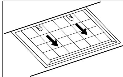
3. Slightly tilt the front of the filter downwards, then pull.
