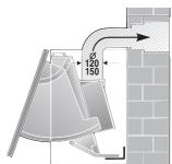
The exhaust air is discharged upwards through a ventilation shaft or directly through the outside wall into the open.
