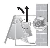
After installing the extractor hood, insert the activated carbon filter.
