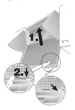
Check that the filter screen is securely located behind the retaining brackets on both sides.
