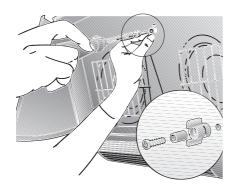
Using a screwdriver or similar, press the two lugs in the housing through to the back (only necessary upon initial fitting).
