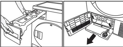
2. Drain the water in the tank.
