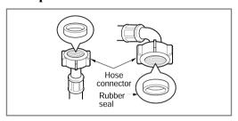
Two rubber seals are supplied with the water inlet hoses.
