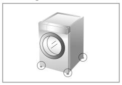
Leveling the washing machine properly prevents excessive noise and vibration. Install the appliance on a solid and level floor surface, preferably in a corner of the room.
