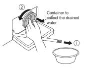
4 After cleaning, turn the pump filter and insert the drain plug.
