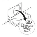
▲ After cleaning, turn the pump filter and insert the drain plug.
