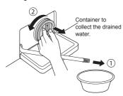
Remove any extraneous matter from the pump filter.
