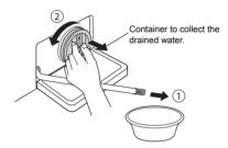
Remove any extraneous matter from the pump filter.
