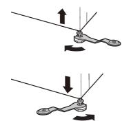
Check if the appliance is perfectly level using a spirit level **①**.
