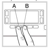
To start the programme press buttons **A** and **B** simultaneously for 5 seconds (see figure). The programme will start automatically and will last approximately 70 minutes. To stop the cycle press the START/PAUSE button.
