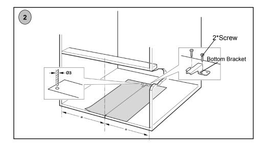
2. Fix the BOTTOM BRACKET with two SCREW. And remove the BOTTOM CABINET TEMPLATE.
