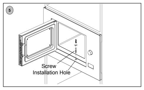
5. Open the door; fix the oven to the cabinet with SCREW at the INSTALLATION HOLE of TRIM KIT. Then fix the TRIM-KIT PLASTIC COVER to the INSTALLATION HOLE.
