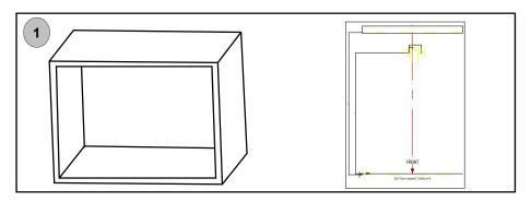
Put the BOTTOM CABINET TEMPLATE on the bottom plane of cabinet.
