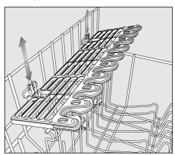
Slide the glass rack to the desired height until the catches click into place at the top or rest on the bottom.
