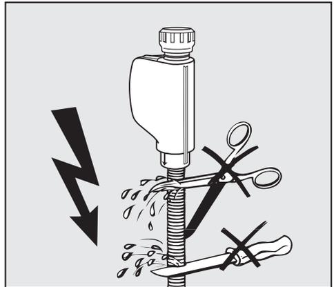
⚠ The inlet hose must not be shortened or damaged in any way as it contains electrical components (see illustration).
