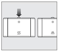
Press the button on the top of the salt reservoir in the direction of the arrow.
